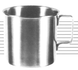
Used in conjunction with AOCS Official Method Ca9a-52 to determine the refining loss of free fatty acids, oil and impurities when the sample is treated with alkali solutions under test conditions. The method applies to crude peanut oil, crude coconut oil, crude corn oil, crude soybean oil (expeller and hydraulic), and crude cottonseed oil (expeller and hydraulic). Cup dimensions: 4 1/2 inch diameter and 4 1/8 inch depth. Capacity: 960 ml.
